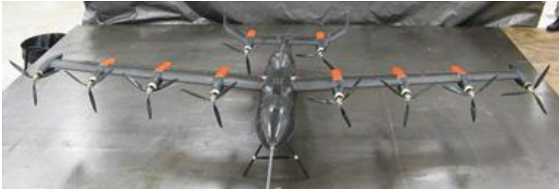
Figure 9: Greased Lightning (GL-10) Distributed Propulsion (DEP) Vehicle flight demonstrator.
