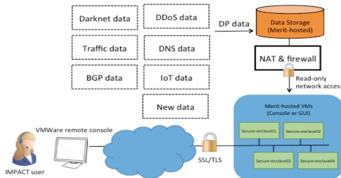
**Figure 4. The secure enclaves data sharing system, hosted at Merit’s cloud infrastructure.**
