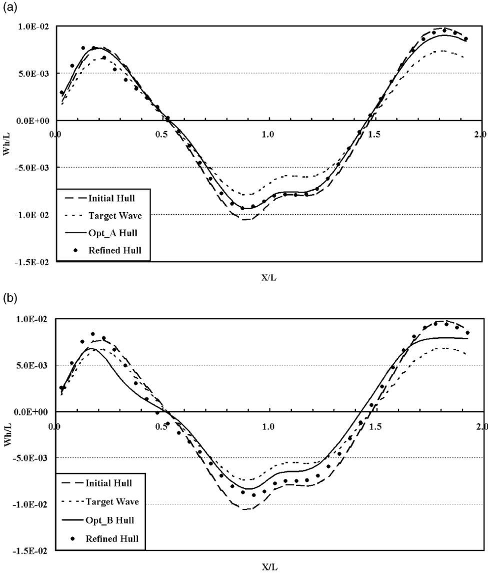
Fig. 12. Comparison of wave profile along catamaran's outside for (a) the initial, Opt\_A and refined hulls and (b) the initial, Opt\_B and refined hulls.
