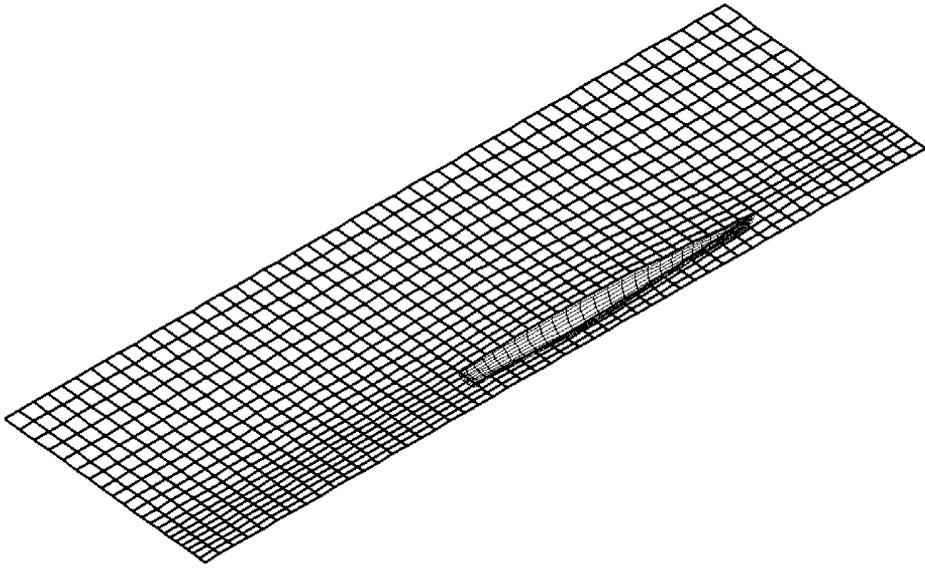
Fig. 1. Penalization example for hull and free surface.
