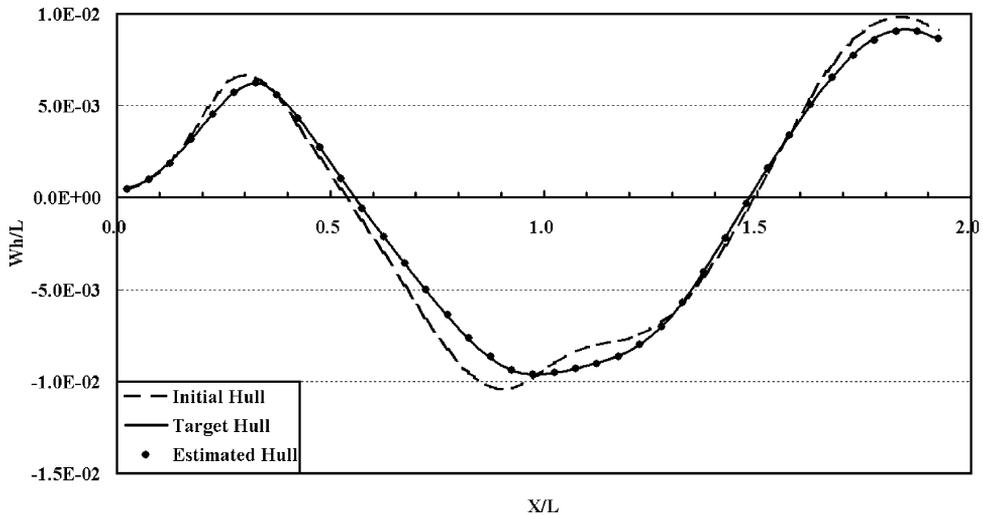
Fig. 7. Comparison of wave cut at 0.14 L off center plane for the initial, target, and estimated hulls using the wave cut data as the inverse design object.
