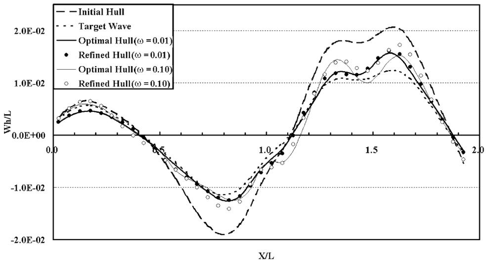
Fig. 8. Comparison of wave profile for the initial, target, optimal, and refined hulls with  $\omega = 0.01$  and 0.10.
