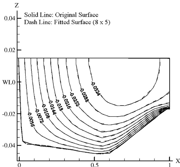
Fig. 2. Buttock plan for the original hull and the fitted surface using  $8 \times 5$  control points.
