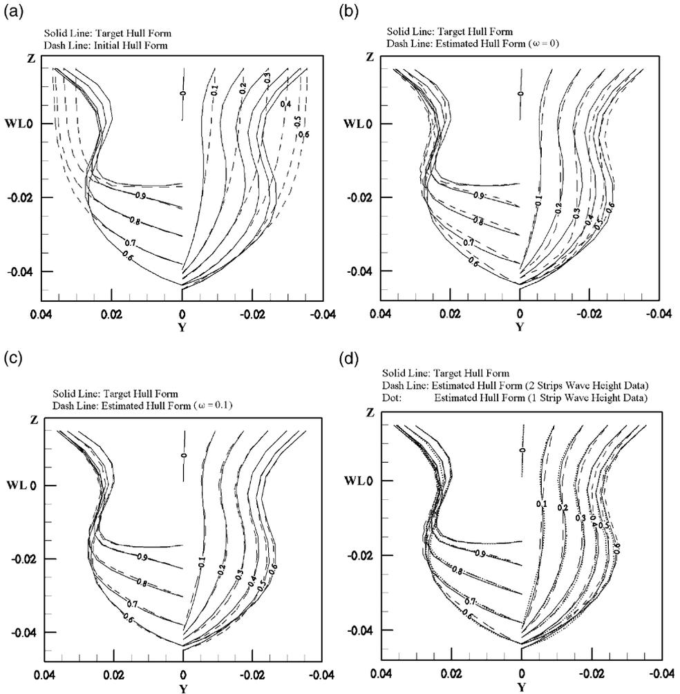
Fig. 4. Body plans for (a) the Initial hull and target hull (b) estimated hulls  $\omega = 0$  (c) estimated hull  $\omega = 0.1$  and (d) estimated hull by 2 strips wave data.
