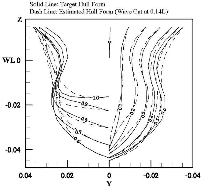
Fig. 6. Body plans for the target and estimated hulls using wave cut data as objective function.
