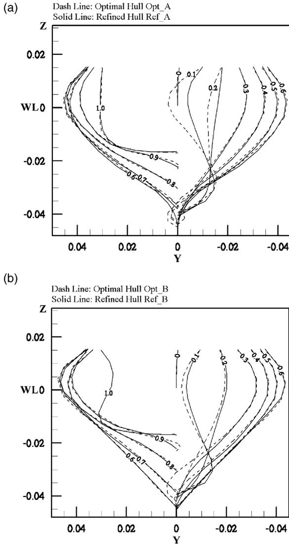
Fig. 13. Body plans for (a) Opt\_A and Ref\_A and for (b) Opt\_B and Ref\_B.
