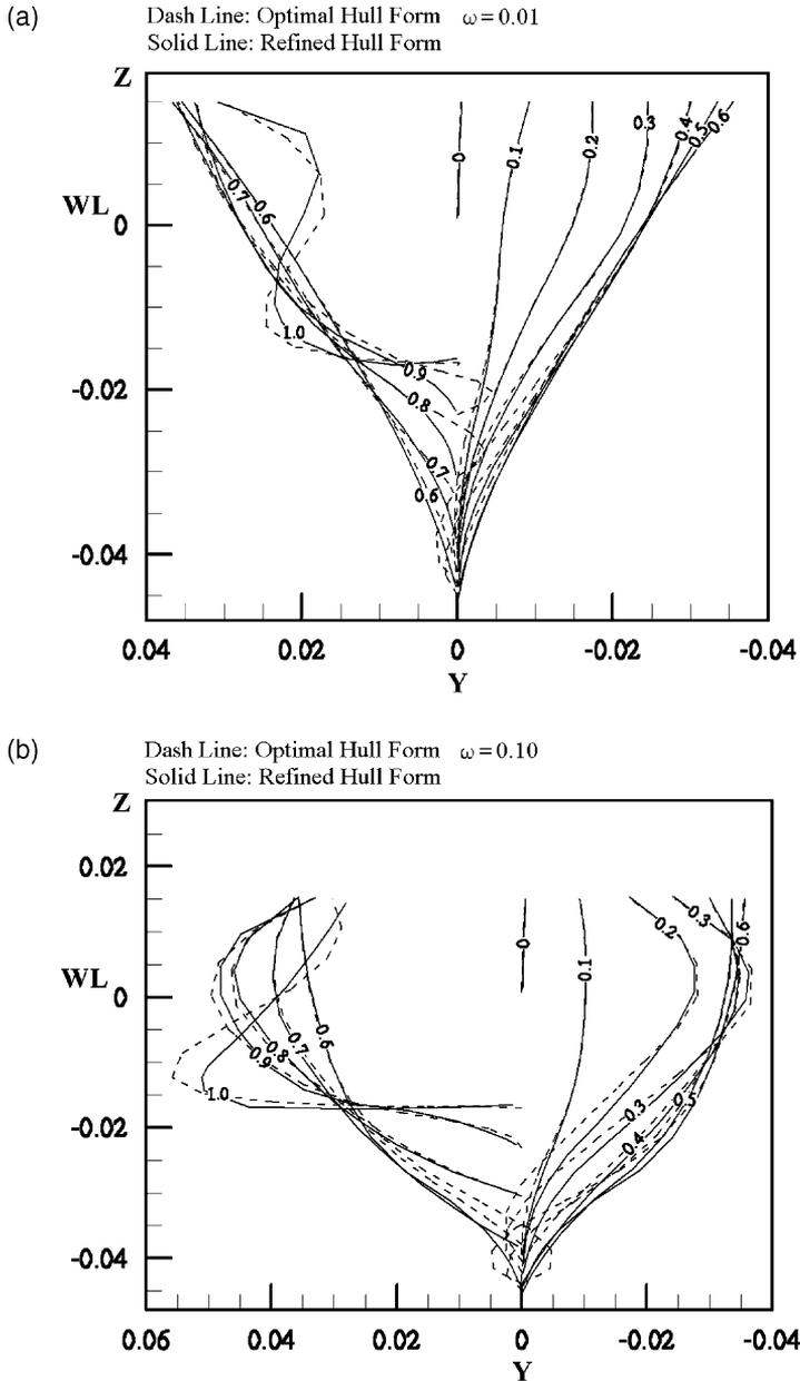
Fig. 10. Body plans for the optimal and refined hulls with (a)  $\omega = 0.01$  and (b)  $\omega = 0.10$ .
