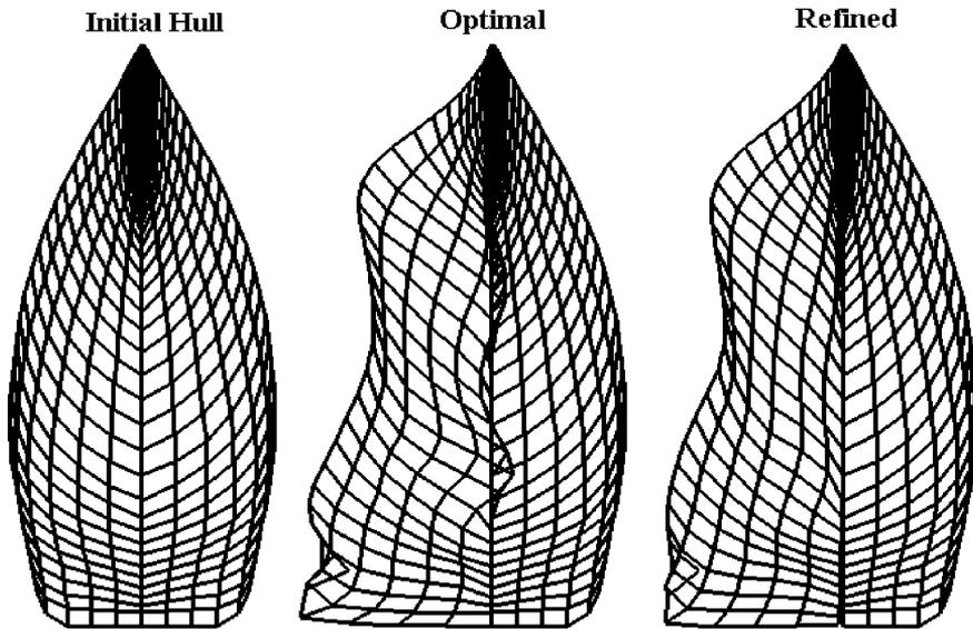
Fig. 9. Comparison of panelized hull forms for initial, optimal, and refined hulls with  $\omega = 0.1$  in Section 6.2.
