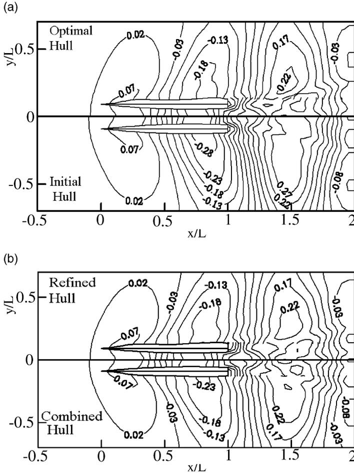
Fig. 11.  $C_p$  plots of free surface for (a). initial and optimal hulls with  $\omega = 0.1$  and (b) refined and combined hulls with  $\omega = 0.1$ .
