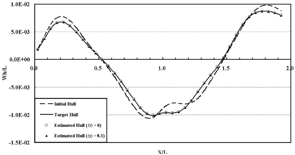
Fig. 5. Comparison of wave profile along catamaran's outside for the initial, target, and estimated hulls for  $\omega = 0$  and 0.1.
