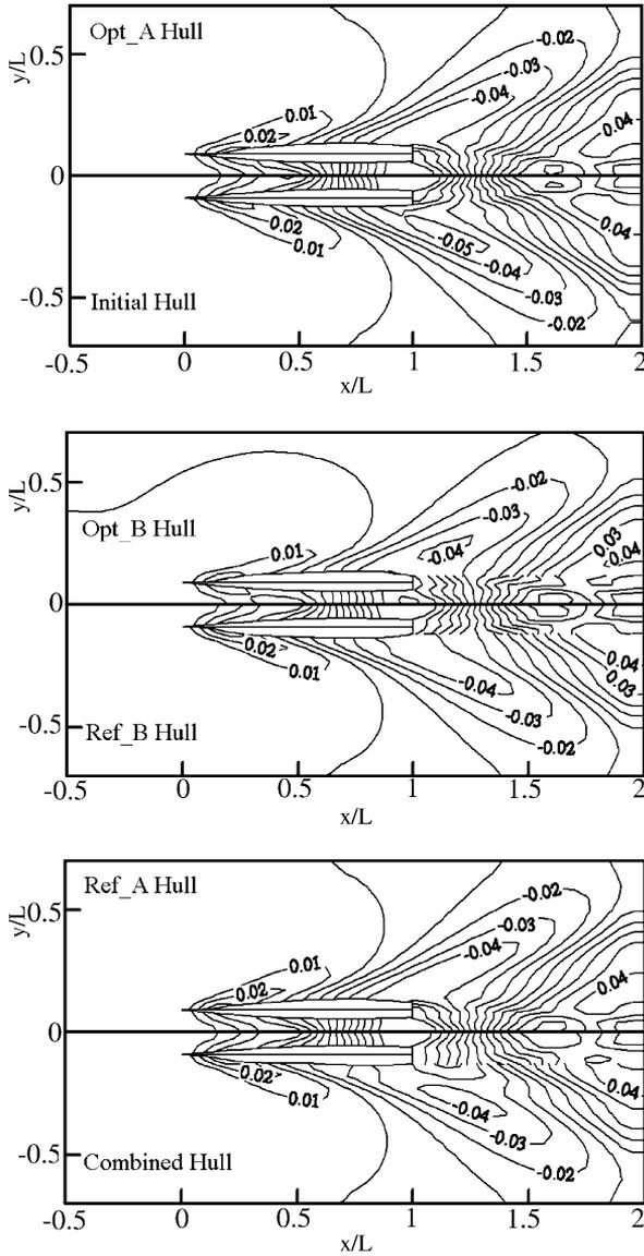
Fig. 15.  $C_p$  plot of free surface (deep-water case  $Fn_L = 0.6428$ ) for the initial, optimal, refined and the combined hulls.
