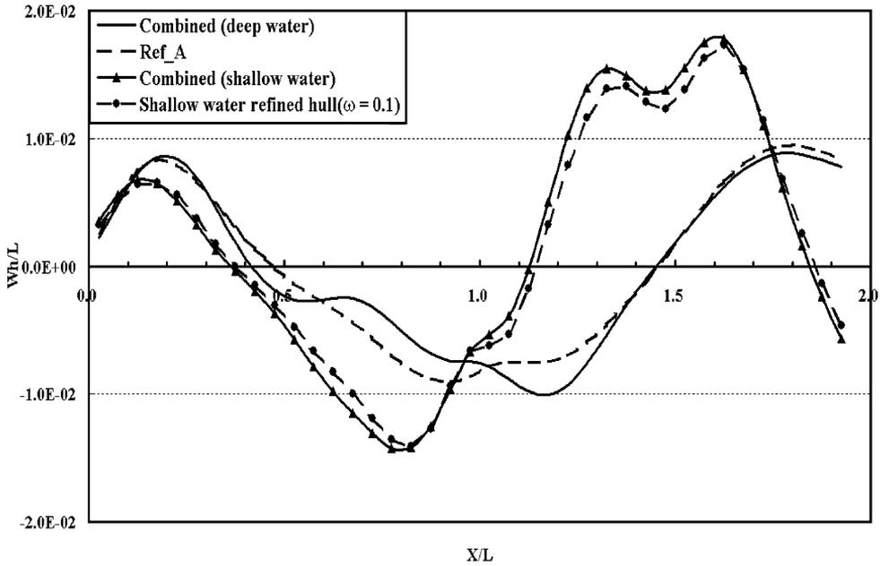
Fig. 17. Comparison of wave profile for the combined hull and the refined optimal hulls at shallow water and deep water.
