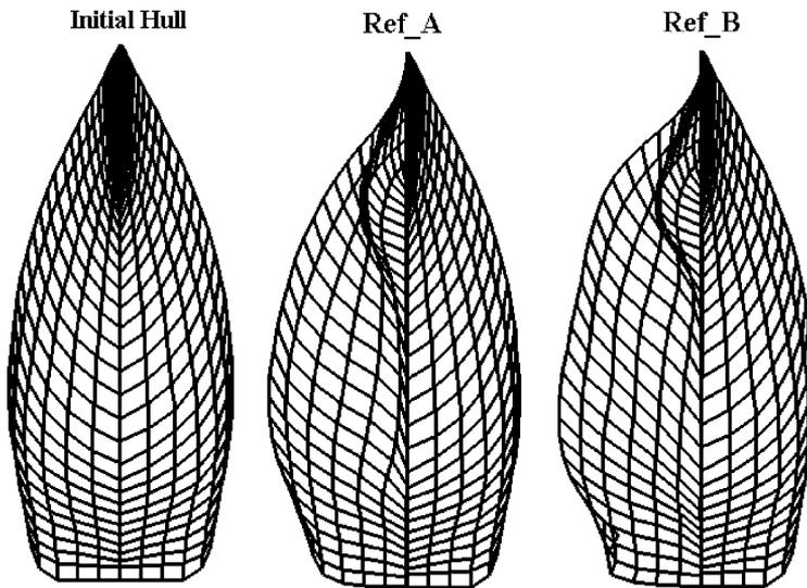
Fig. 14. Comparison of panelized hull form of Section 6.3 for the Initial, Ref\_A, and Ref\_B hulls.
