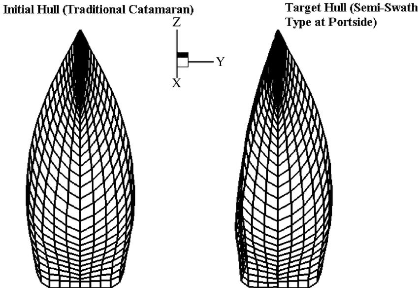
Fig. 3. Panelized hull for Initial and target hulls used in Section 6.1.
