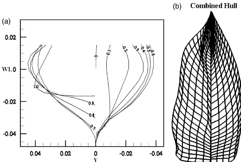
Fig. 16. (a) Body plan and (b) panelized hull form for the combined hull form.
